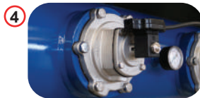
MEMBRANE ELECTRO VALVE: two way valve normally closed; it is activated by an electric solenoid. It holds air pressure of max. 6 bar. The compressed air tank operates at 4 to 6 bar.
